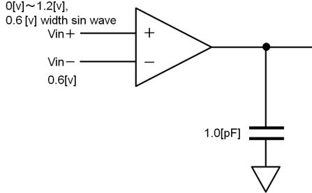
Fig. 13. The circuit for DC gain verification
