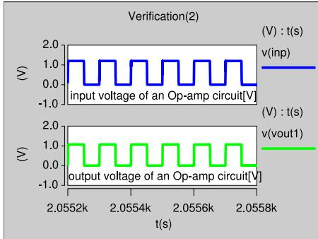
Fig. 18. Verification (2):Transition of the input-and-output voltage of an op-amp circuit
