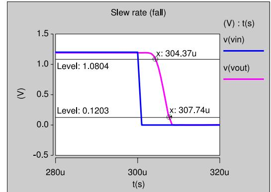
Fig. 12. Slew rate verification (fall)
