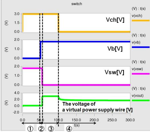
Fig. 6. Virtual power supply wire voltage for parameter settings
