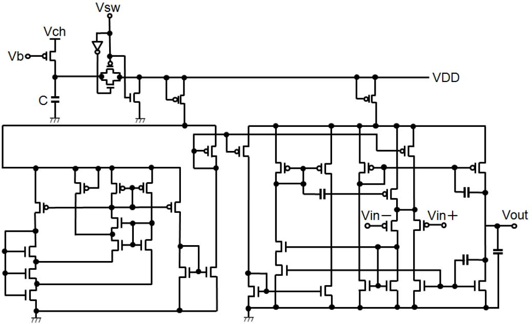
Fig. 7. The whole proposed system circuit diagram with the supply plug PMOS
