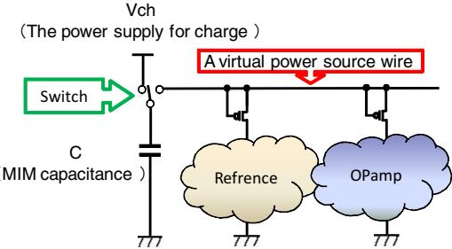
Fig. 4. The structure of our proposed system
