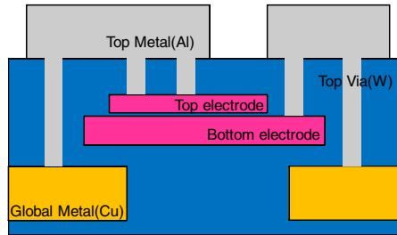
Fig. 1. The sectional view of MIM-type capacitor
