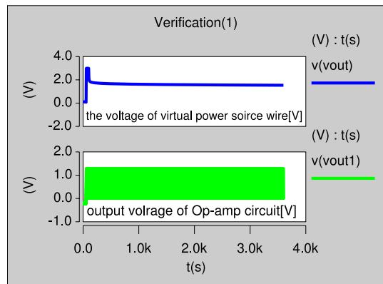
Fig. 15. Verification (1):Transition of the voltage of a virtual power supply wire, and the output voltage of an op-amp circuit
