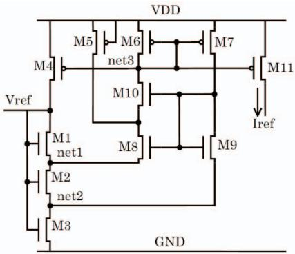
Fig. 3. nA reference circuit
