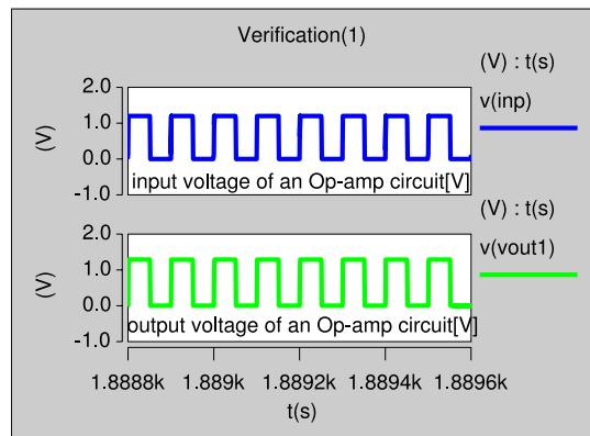
Fig. 16. Verification (1):Transition of the input-and-output voltage of an op-amp circuit
