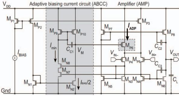
Fig. 2. Op-amp circuit with adaptive biasing
