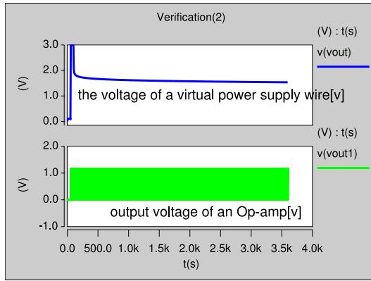
Fig. 17. Verification (2):Transition of the voltage of a virtual power supply wire, and the output voltage of an op-amp
