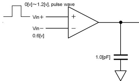
Fig. 10. The circuit for slew rate verification
