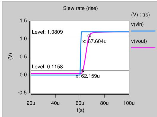
Fig. 11. Slew rate verification (rise)
