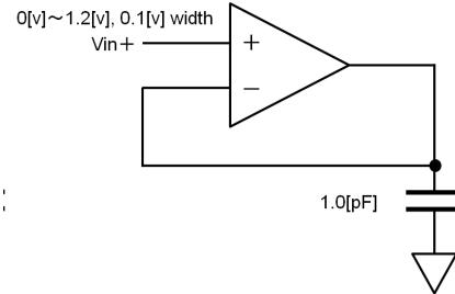
Fig. 8. The circuit for input dynamic range verification
