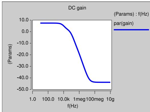
Fig. 14. The verification result of a low gain op-amp
