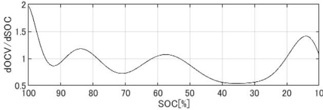
Fig. 4. The gradient of the OCV curve
