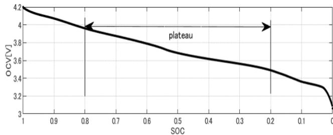
Fig1. OCV-SOC curve
