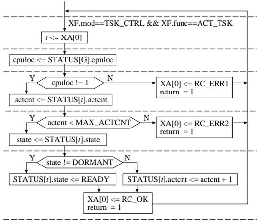
Fig. 10. RTL behavior for task activation
