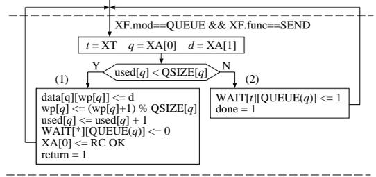
Fig. 8. RTL behavior of data queue module (send)
