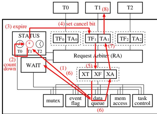
Fig. 11. Mechanism of timeout
