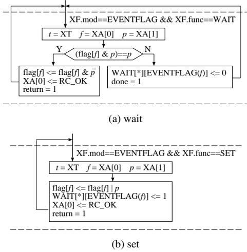
Fig. 6. RTL behavior of eventflag module
