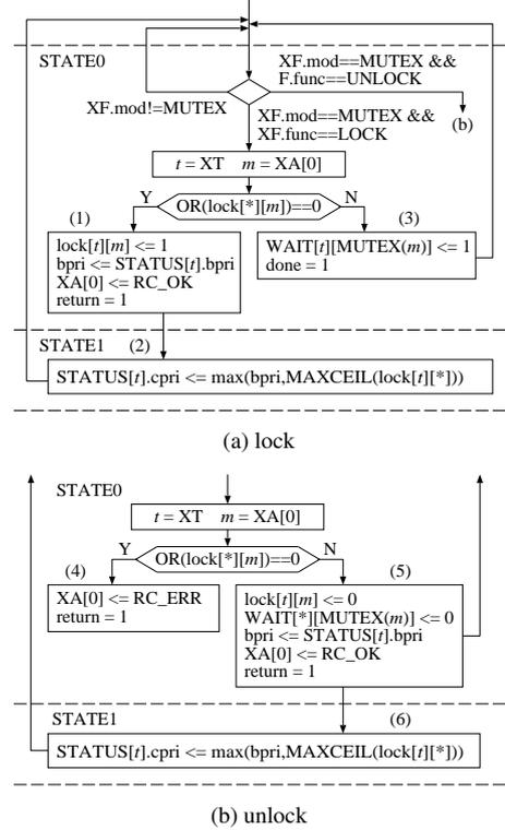
Fig. 5. RTL behavior of mutex module
