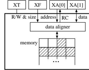
Fig. 9. Shared variable read/write module
