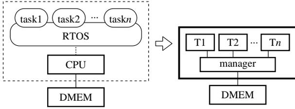
Fig. 1. full hardware implementation of RTOS-based system [12]
