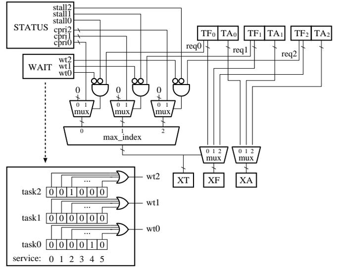
Fig. 3. Hardware configuration of request arbiter (RA)
