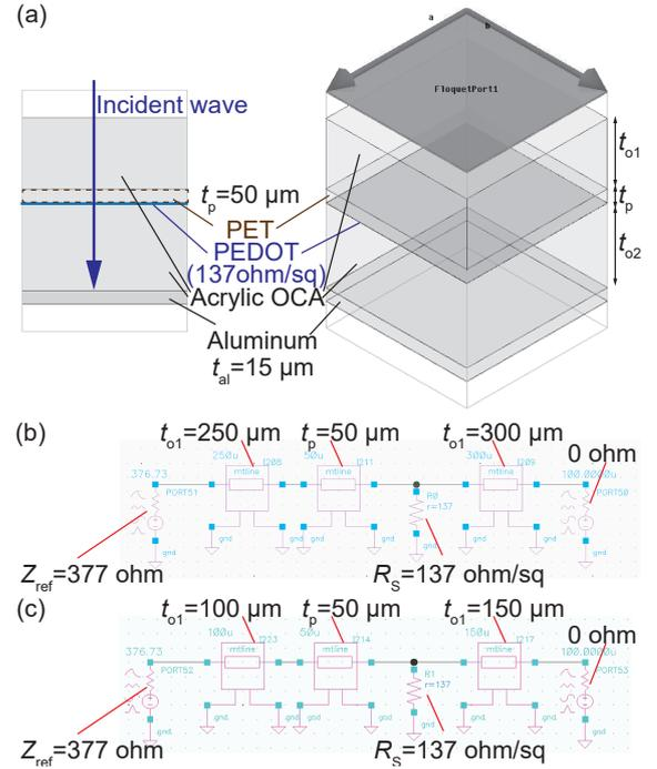
Fig. 6. (a) An EM-simulation model for fabricated absorbers [2]. Proposed simulation models based on *RLGC* parameters: (a) Absorber 1(150-GHz band) [2], and (b) Absorber 2(300-GHz band) [3].
