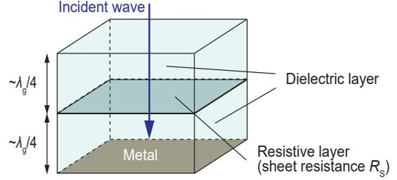
Fig. 3. Jaumann-type EM-wave absorber [2, 3].
