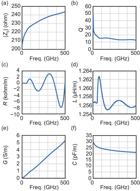
Fig. 2. Transmission-line parameters of a dielectric (acrylic OCA): (a) Characteristic impedance, (b) quality factor. Parameters per length: (c) Resistance, (d) inductance, (e) conductance, and (f) capacitance.
