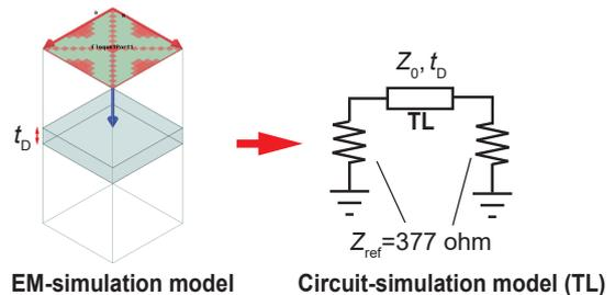
Fig. 1. Simulation-model conversion.
