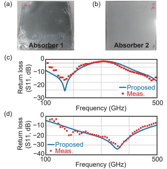
Fig. 7. Fabricated absorbers for (a) Absorber 1 [2], and (b) Absorber 2 [3]. Comparison between simulation and measurement results: (c) Absorber 1, and (d) Absorber 2.
