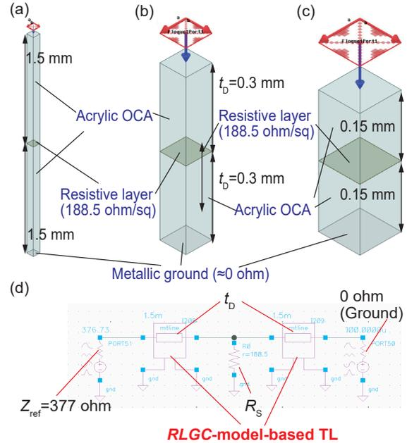
Fig. 4. EM-simulation models based on a Jaumann-type EM-wave absorber for (a) 30-GHz, (b) 150-GHz, and (c) 300-GHz frequency bands. (d) Proposed circuit simulation model using Cadence Spectre (components (port, mtline, res, gnd) were imported from the library of AnalogLib).
