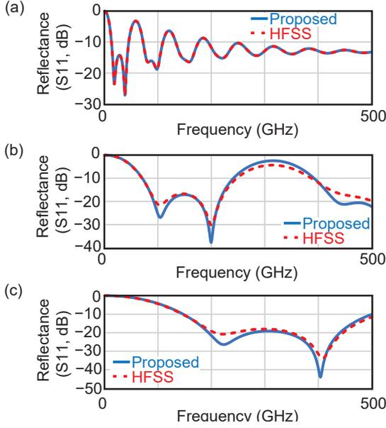
Fig. 5. Result comparison: (a)  $t_D = 1.5$  mm, (a)  $t_D = 0.3$  mm, and (c)  $t_D = 0.15$  mm.
