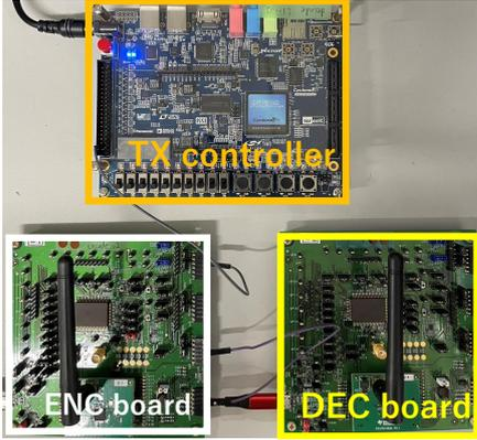
Fig. 4. Operation Confirmation Environment. The FPGA at the top center is the TX controller. The EVM at the bottom left is the ENC board. The EVM at the bottom right is the DEC board.
